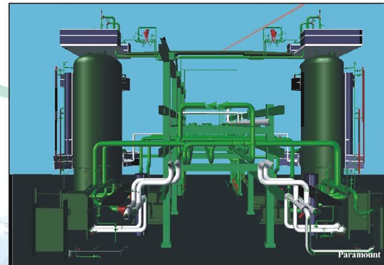
De-Hazing / Moisture Control System at Kuwait Refinery
