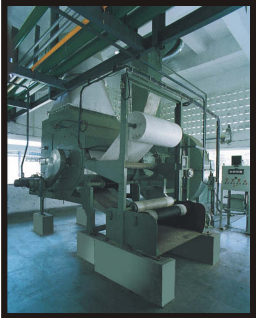
Rotary Drum HEAF™ Unit for Plasticizer operation
