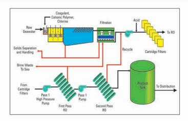
Sea water from its intake facility (after pump house) is screened of large solid matter prior to pre-treatment for removal of suspended solids and correction of pH.
