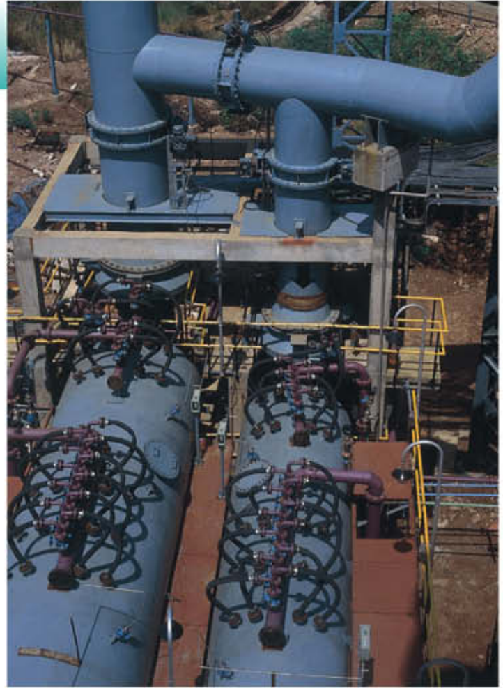
A view of SO 2 Scrubber at a Copper smelter
